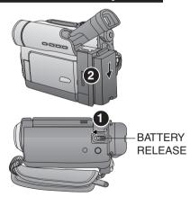
While sliding the BATTERY RELEASE, slide the Battery downward and remove.
