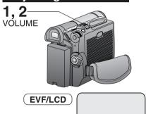
Slide VOLUME to adjust the volume of the built-in speaker in PLAY mode.
