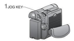
During Still mode, **rotate JOG KEY** to advance or reverse the picture one frame at a time.
