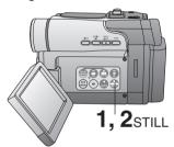
While in RECORD mode, **press STILL** to capture a still picture. The captured still picture will be recorded together with sound.
